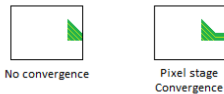
Figure 5.3.e. Diagram showing the convergence shift applied at the pixel stage, resulting in artefacts.
